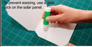
3. Fold the **solar panel**. Then use a glue stick to apply a very thin layer of glue on one inside half and glue the sides together. Wrap it in wax paper, and press it in a heavy book overnight. (For additional strength, trace one half of the panel on a blank piece of card stock. Cut it out and layer it inside the folded panel before you glue it together.) AFTER the glue dries, trim the panel.
