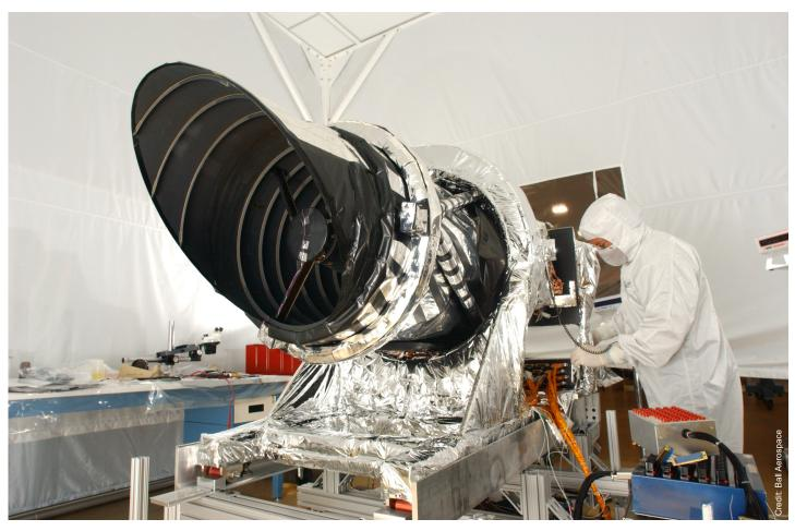
The Ball-built HiRISE telescope flies onboard the Mars Reconnaissance Orbiter (MRO) spacecraft, which NASA launched in 2005. As MRO orbits Mars, HiRISE images wide swaths of its surface.
