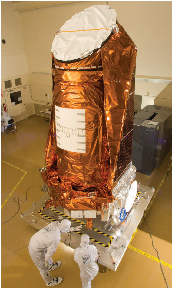
The Kepler Space Telescope is part digital camera and part light meter (photometer). It measured the dip in light that occurs when a planet transits its star.
