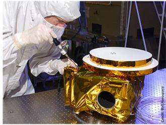
The Ball-built Ralph camera took color images of Pluto and mapped its surface, atmosphere and temperature.
