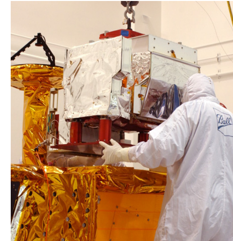
11 Crosstrack Infrared Sounder (CrIS)
