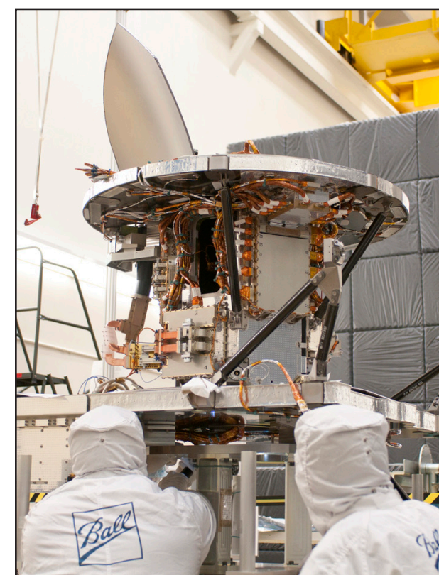
6 Mounting Cold Sky Reflector on Instrument Base Structure
