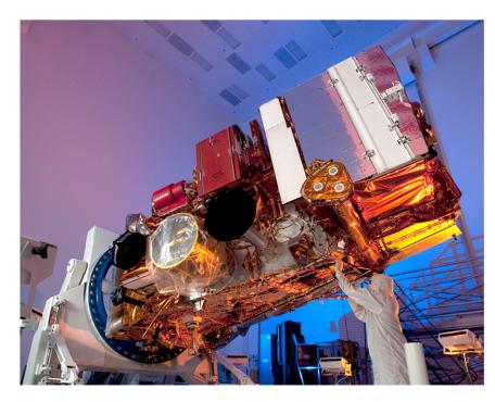
Suomi NPP was the first of a new generation of weather satellites. Ball designed and built the bus, which enables the satellite's five instruments. Ball also built OMPS, the instrument that measures our atmospheric ozone. Launched in 2011, the spacecraft orbits 512 miles above Earth.
